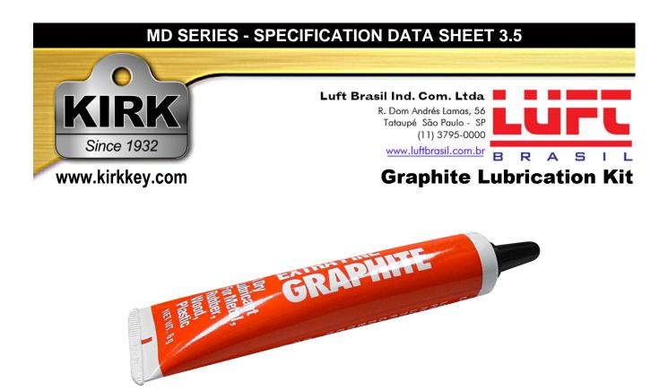
MD Series interlocks should be periodically lubricated with a small amount of dry powdered graphite. Do not use oil of any type as the oil will collect dirt and "gum up" the lock cylinder so that it will not operate.
